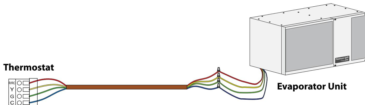
**NOTE:** To ensure correct system operation, the 24V thermostat must be placed inside the wine cellar, preferably in a central location away from any airflow.
