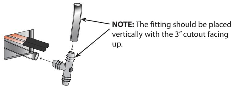
**NOTE:** The fitting should be placed vertically with the 3" cutout facing up.
