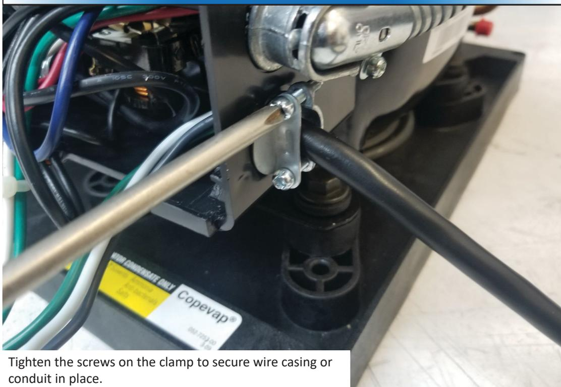
Tighten the screws on the clamp to secure wire casing or conduit in place.
