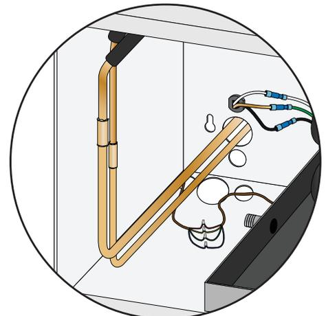
11. Remove the line set caps. Route the 3/8" suction line and 1/4" liquid line into the unit and braise.
