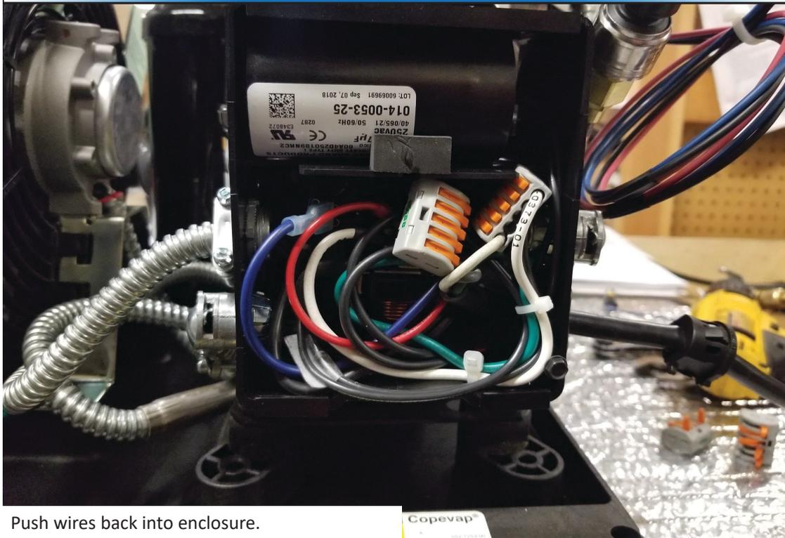
Push wires back into enclosure.
